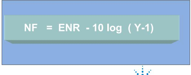
**Y = Np (on) / Np (off) =** change in detected power level as source switches from Tc to Th
